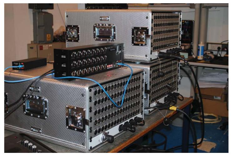
Sony needed interchangeable, removable lids on each end of the cases and racks. All of CP Cases broadcast cases are handmade and due to the nature of the 2mm rigidised aluminium used, there can be a fraction of a mm difference between each case. It requires a great deal of skill and experience of working with this material to achieve the required accuracy, something CP Cases have in abundance.
